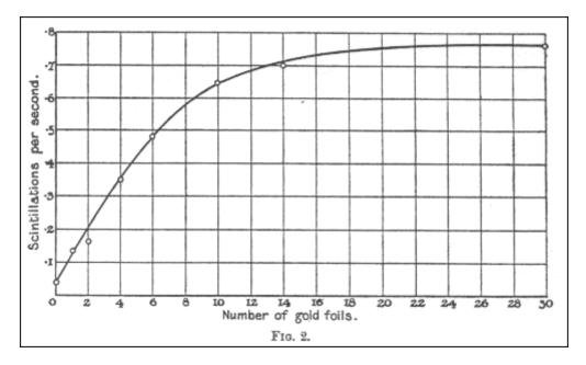
The curve is similar to those which have been obtained for the reflection of the  $\beta$ -particles.\* It brings out clearly that the reflection is not a surface but a volume effect.
