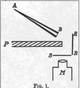
with radium emanation, the end B of the tube being closed airtight by means of a mica window. The thickness of the mica was equivalent to about 1 cm. of air, so that the  $\alpha$ -particles could easily pass through it.
